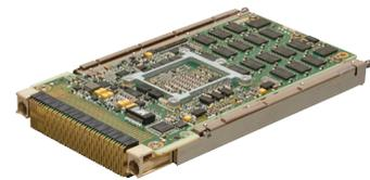
Typically, processors throttle back at high temperatures, reducing performance. The SBC347D has an innovative cooling architecture that enables it to maintain 100% of its rated performance even at 75°C.
